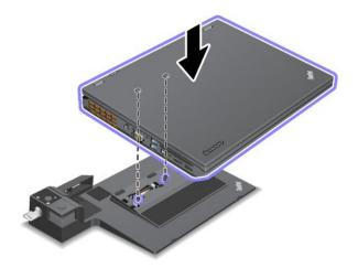
4. Insert your computer into the docking station until you hear a click. The computer is attached to the docking station.
